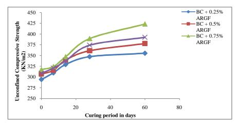
Fig. 4 Variation of UCS for BC soil with various percentage of ARGE fibres
