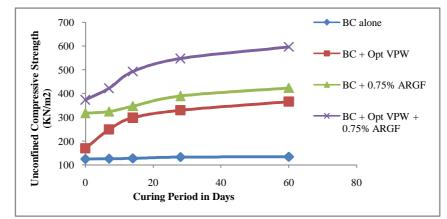
Fig. 7 Comparison of UCS of BC Soil Alone, BC +15% VPW, BC+ 0.75% ARGF and BC Soil +15% VPW+ 0.75% ARGF.
