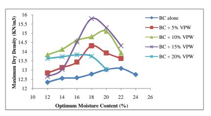
Fig.3 Compaction characteristics of BC soil with varying percentages of VPW
